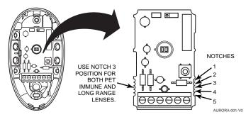
Figure 7. PCB Vertical Adjustment for Lenses
